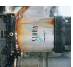
Corrosion Test (In seawater / 1 month)
